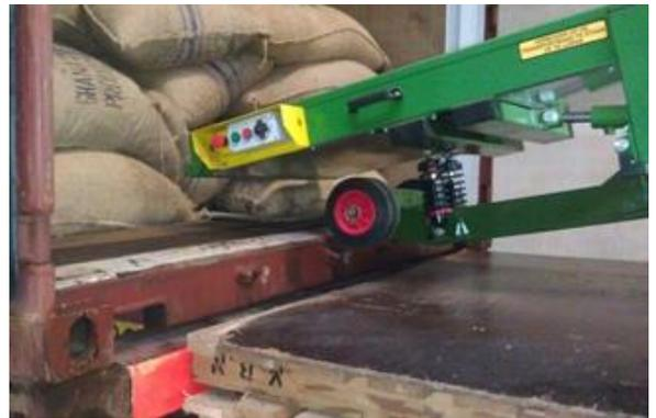
Drop snout on front side of the pewiSYS/Newland MTC™
